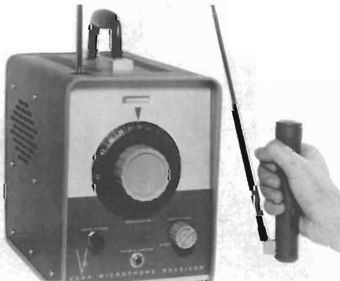
Fig. 1. This "Vega-Mike" system is typical of the high-quality wireless microphones licensed to operate on commercial bands.
