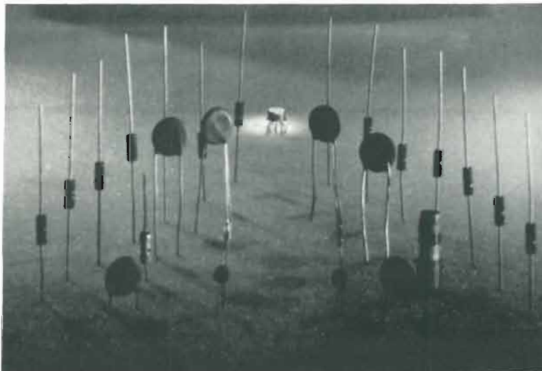
Fig. 1. The linear IC (in spotlight) replaces 26 components shown, besides the many soldering points formerly required.
