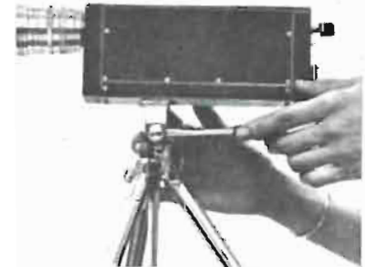
TINY TV CAMERA for space and military use is one of the miracles of integrated circuitry. This one weighs 27 ounces, uses a one-inch vidicon camera tube, and requires only four watts of power.
