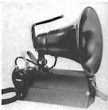
Fig. 1. (Left) This 25-watt semi-portable power megaphone has a detachable microphone and range of one mile. (Center) Hand-held, lightweight, one-watt unit has range of 150 yards. (Right) 16-watt "bullhorn" has range in excess of 800 yards.
